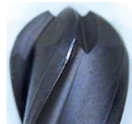
IDI diamond tool: after 10500m cutting length
