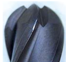
IDI diamond tool: after 10500m cutting length
